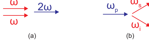
Figure 2.4: Feynman diagrams for second-order nonlinear processes. (a) Second harmonic generation or frequency doubling. Two pump photons of the same frequency \omega get annihilated producing an output photon of frequency 2\omega . (b) Down-conversion. A pump photon of frequency \omega_p gets annihilated producing two photons at the signal and idler frequencies \omega_s and \omega_i , respectively. The sum of the signal and idler frequencies \omega_s and \omega_i is equal the pump photon frequency \omega_p .
