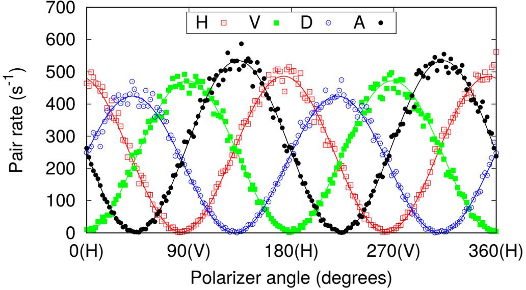
Figure 2.7: Polarization correlation in both H/V and D/A bases measured at the entanglement source. The coincidence rate is measured with two polarizers applied to the signal and idler photons. The polarizer on the signal’s side is kept at different settings (H, V, D, A), while the other polarizer on the idler’s side is scanned over 360 degrees.
