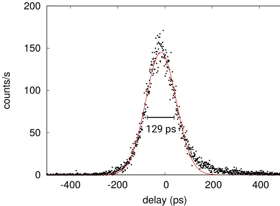
Figure 2.12: An exemplary cross-correlation histogram obtained by detecting signal and idler photons with two commercial InGaAs APDs (ID220 APD module from IDQuantique). The coincidence peak is fit to a Gaussian distribution with a standard deviation  $\sigma = 64.5$  ps. If one assumes an identical performance between the two detectors, then they each have a standard deviation in timing jitter of 45.6 ps.
