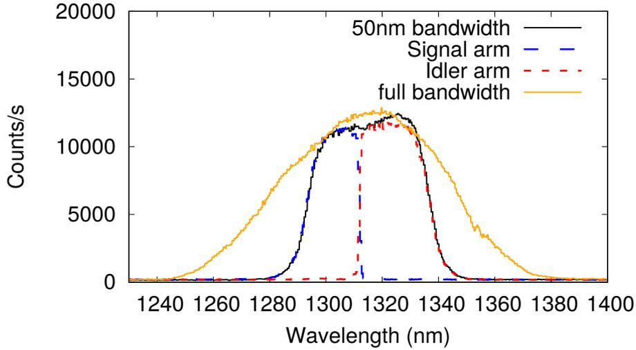
Figure 2.4: Spectrum of the Type-0 SPDC photons. The orange trace shows the full spectrum of the SPDC photons and the black trace indicates the 50 nm bandwidth defined by the bandpass filter applied. Signal (blue) and idler (red) photons are separated using a wavelength division demultiplexer edged at 1316 nm.
