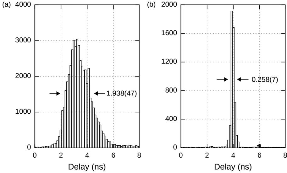
Figure 4.7: Timing correlation of photon pairs propagating in deployed telecommunication fibers.
