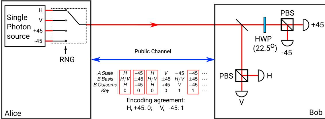
Figure 1.2: An illustration of the BB84 protocol: Alice randomly prepares a photon in one of the 4 polarization states (H, V, +45, -45) and sends it to Bob; Bob randomly measures the photon’s polarization in one of two bases (H/V, +45/-45). After a series of measurements, Alice and Bob inform each other of the basis choices made for each generated/detected photon to establish a secret key. A Random Number Generator (RNG) is used to ensure randomness in state preparation.
