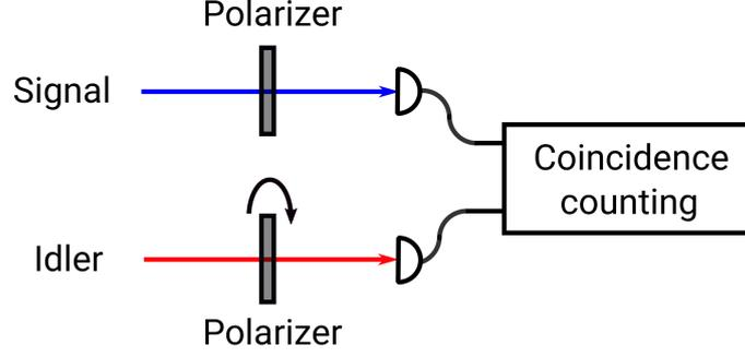
Figure 2.6: Setup for measuring the polarization correlation of the entanglement source in both H/V and D/A bases. The coincidence rate is measured with two half-wave plates (HWPs) and two polarizing beam splitters (PBSs) applied to the signal and idler photons. The HWP on the signal's side is kept at different polarization measurement settings (H, V, D, A) while the other HWP on the idler's side is scanned over 180 degrees.
