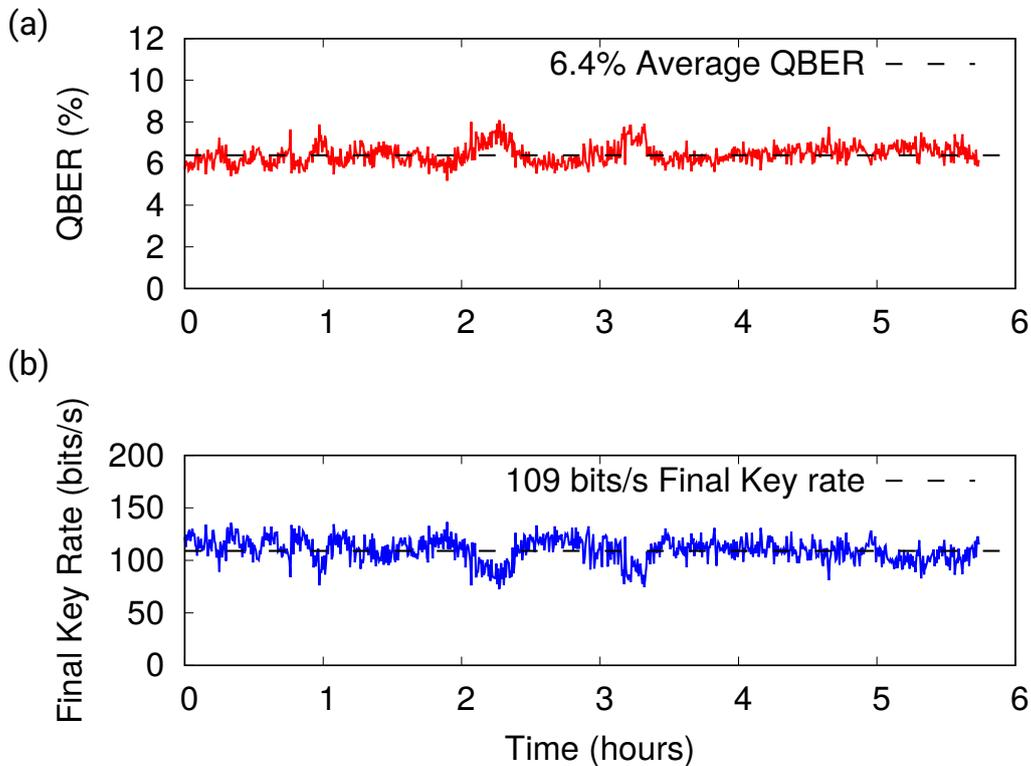
Figure 5.9: QBER (a) and final key rate (b) logged over 5.7 hours of continuous operation. Error correction and privacy amplification are performed over blocks of raw key bits integrated over 25 seconds. Data collection stopped after 5.7 hours due to a detector failure.
