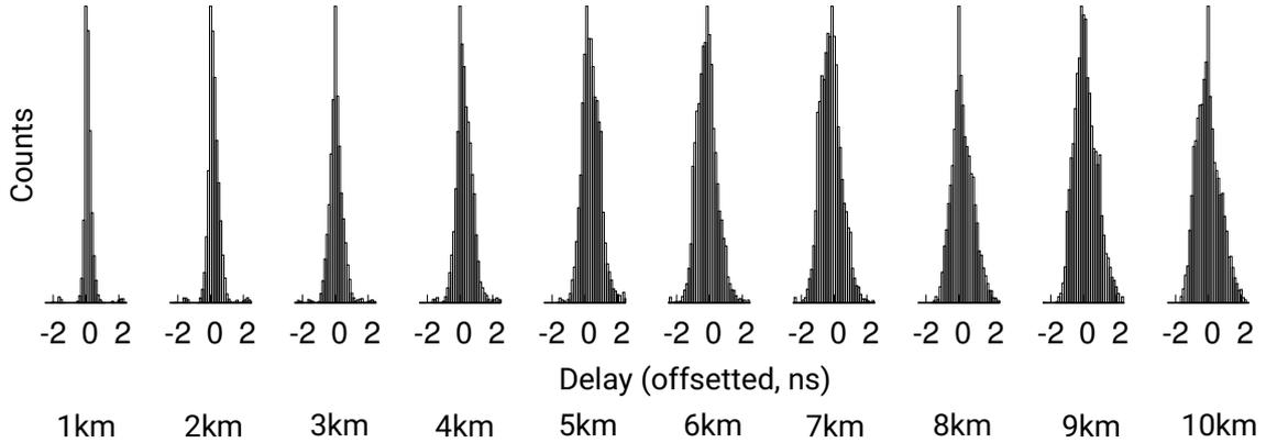
Figure 4.2: Timing correlation of photon pairs with only one of the photons propagates through a long fiber with lengths varying from 1 km to 10 km. The delay in the time of flight in fiber is offset to zero and the count rates in different measurements are normalized to the same height for easier comparison of the coincidence width.
