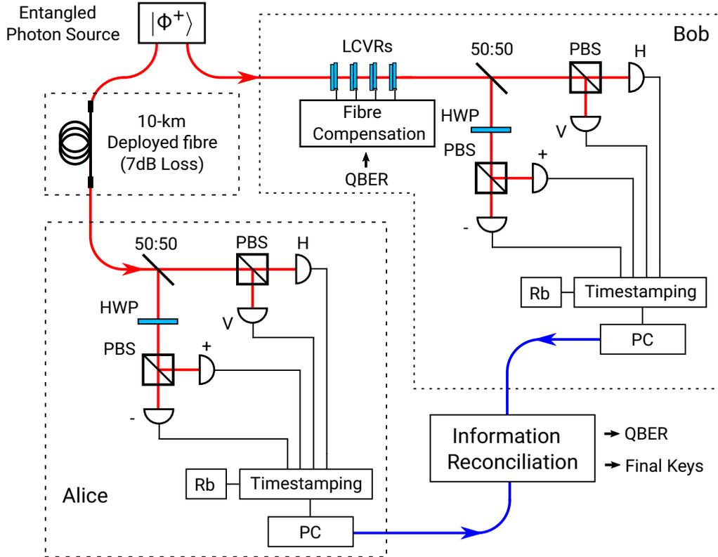
Figure 5.7: QKD setup over 10 km deployed fiber link. The fiber loops back to the lab to simplify the experimental procedure. The Alice and Bob nodes are run on independent clocks. Alice's analyzer is connected to the entanglement source via the 10 km deployed fiber while Bob's setup is locally connected using a short patch cord. The two hosting PCs are connected to the same local area network in order to exchange timestamp data for coincidence identification.
