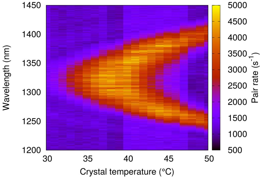
Figure 2.3: Measured SPDC spectrum as a function of crystal temperature. In this source setup, the PPKTP crystal temperature is stabilized at 40 °C where the signal and idler wavelengths are degenerate and the brightness is the highest.
