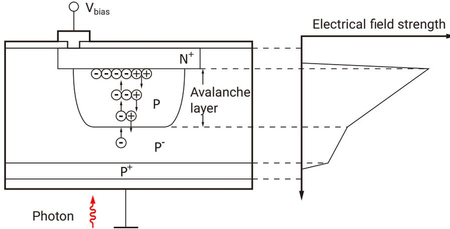
Figure 2.8: A simplified diagram illustrating the avalanche process in an APD. A high bias voltage is applied to the APD which creates a depletion region in the weakly doped  $P^-$  and  $P$  region. A single photon incident on the APD creates a free electron-hole pair, which then triggers an avalanche. The number of free charge carriers quickly multiplies in the avalanche layer and eventually forms a measurable amount of electrical current. This diagram is adopted from reference [77].
