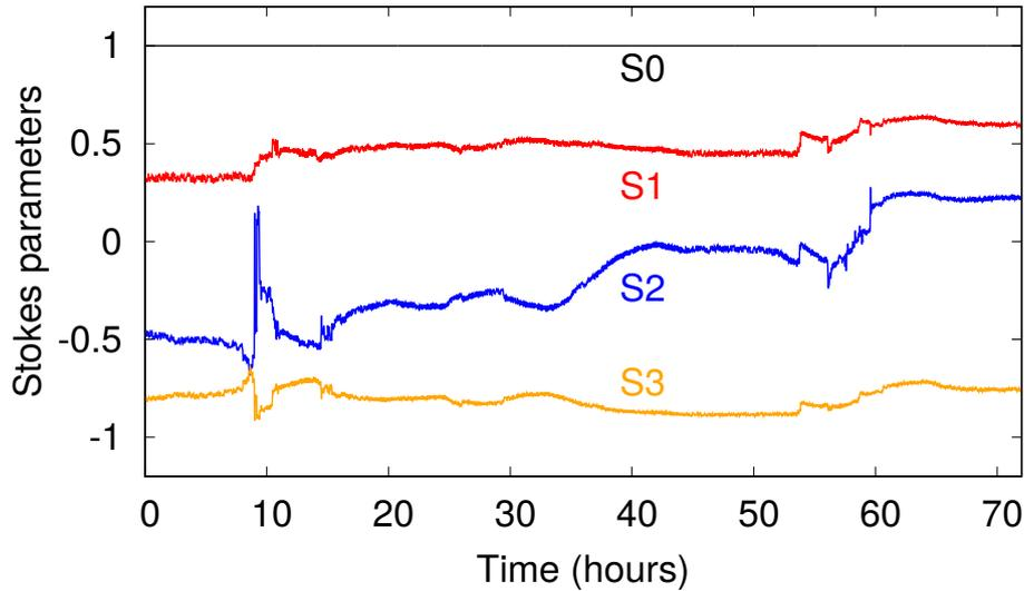
Figure 5.3: Stokes parameters of polarisation state at the fiber output logged over 3 days showing drifts on a time scale of days. The measurement setup is the same as the one shown in Fig. 5.2 (a) with the laser wavelength kept constant at 1310 nm. The measured polarization drifts slowly for the majority of time with sudden jumps occurring occasionally.
