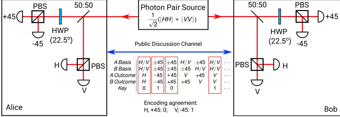
Figure 1.3: An illustration of the BBM92 protocol: An entanglephoton pair source distributes photons to Alice and Bob. The photon pairs are prepared in a polarization entangled state  $\frac{1}{\sqrt{2}}(|HV\rangle + |VH\rangle)$ , and are randomly measured in one of two bases (H/V, +45/-45) on both sides. The measurement results between Alice and Bob are correlated and can be used to establish a secret key composed of random bits.
