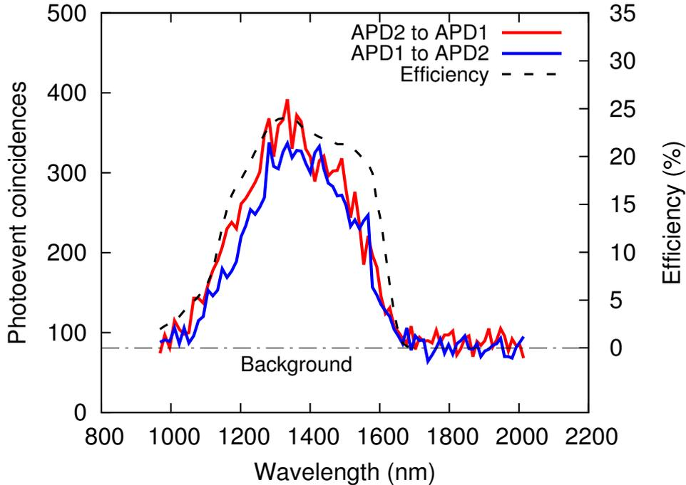
Figure 3.5: Spectral distribution of the InGaAs APD breakdown flash. The integration time for each data point is 30 minutes. We record cases where APD1 emits a breakdown flash that is detected by APD2 and vice versa. The two spectra range from 1000 nm to 1600 nm and peak at about 1300 nm. The dashed line indicates the background due to accidental coincidences.
