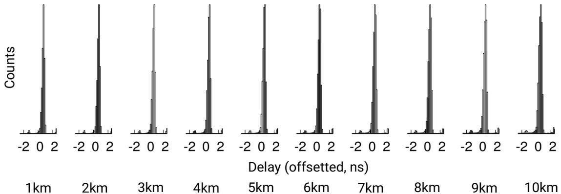
Figure 4.5: Timing correlation of photon pairs with both photons propagating through the same fiber with varying lengths. The timing correlation is much better preserved over these distances as compared to the previous case (Fig. 4.2)
