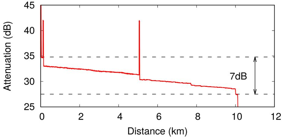
Figure 5.8: Optical time-domain reflectometer trace of the deployed fiber, identifying a high reflection loss point about 5 km away from both endpoints. Two more points with high reflection/absorption loss are also identified about 100 meters from the endpoints, which is due to a patching cable between the deployed fiber and the laboratory setup.
