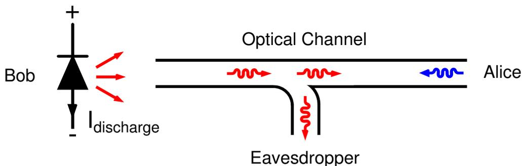
Figure 3.1: A single photon carrying information on phase or polarization is sent from Alice to Bob. The detection of the photon triggers breakdown flash which is partially coupled back into the fiber channel, giving Eve access to the timing and/or polarization information of the detected photon.
