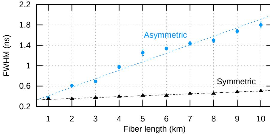
Figure 4.6: Cross-correlation peak width (FWHM) for photon pairs after propagating through various lengths of SMF28 fiber. In the asymmetric case where one photon is detected locally with a negligible amount of chromatic dispersion while the other photon travels through different fiber lengths, the FWHM increases with lengths with a slope of 167 ps/km. In the symmetric case where both photons propagate through the same fiber length, this slope is reduced to 18 ps/km.
