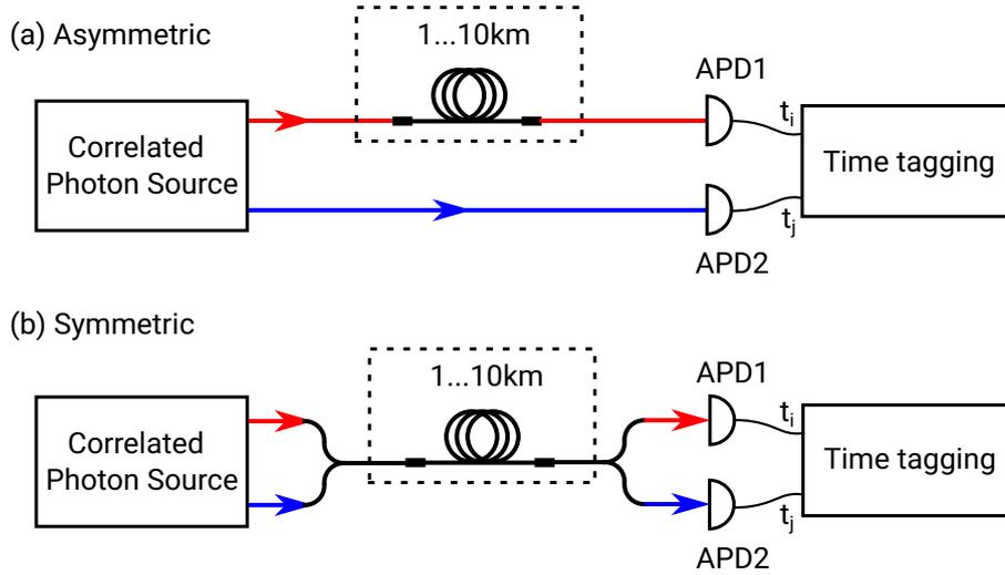
Figure 4.1: Experimental setup for measuring the timing correlations of photon pairs propagating over long fibers. In the asymmetric configuration (a), one of the photons is transmitted through a long fiber while the other photon is detected locally. In the symmetric case (b), both photons are sent through the same long fiber and are only separated after fiber transmission. Both measurements are repeated with different fiber lengths ranging from 1 km to 10 km.
