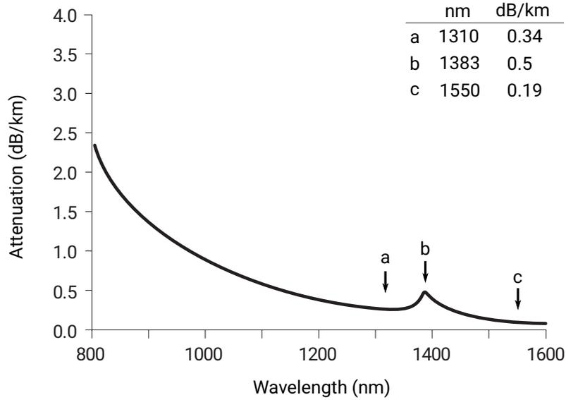
Figure 2.1: Attenuation spectrum of a typical SMF-28 fiber. There are two commonly used transmission windows located at 1310 nm (a) and 1550 nm (c), separated by a high loss peak around 1383 nm (b) caused by hydroxyl ( $\text{OH}^-$ ) ion absorption. This figure is adapted from reference [54].
