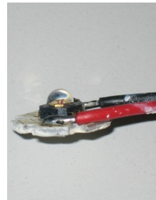
(c) A picture of the Luxeon K2 LED side view, showing the plastic cap.
