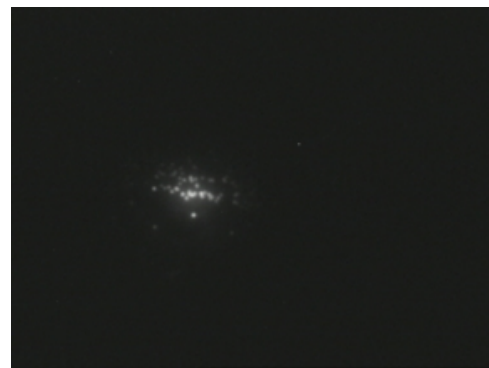
(b) Picture of laser illuminated Fluorescent beads by decreasing the laser radiant flux to give the same level of fluorescence as the LED picture in Figure 54(a). Note the same bead pattern in the same illuminated area in Figure 54(b).
