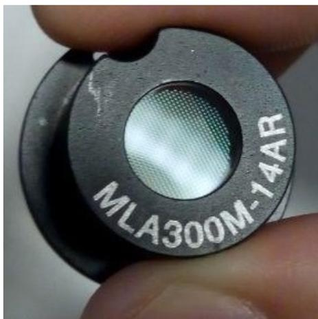
Figure 3.1: A photograph of the lenslet array that can be affixed onto the CCD camera. The green dots on the optical element is the lenslet array reflecting the lighting in the laboratory
