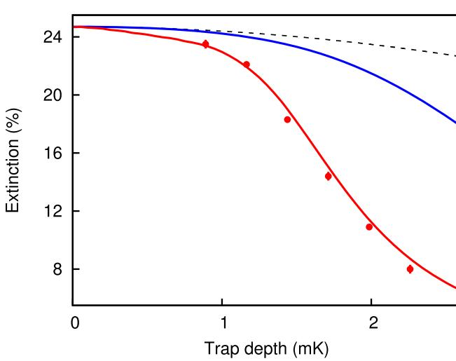
**Figure 4.** Resonant extinction for various trap depths. Red circles: measured extinction, red line: full 12-level numerical simulation, black dashed line: first order approximation  $\epsilon_0 \eta_{\text{dme}}^{(1)}$  (equation (11)), blue line: numerically calculated  $\epsilon_0 \eta_{\text{dme}}$ .
